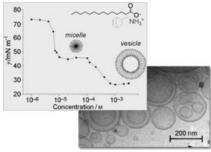
Micelles or Vesicles? Single-tailed surfactants have been associated with various organic counterions. Depending on the structure of the ion-paired surfactant, a micelle-to-vesicle transition is observed (see picture), thus demonstrating the key role played by the positioning of the counterion in supramolecular self-assembly.
